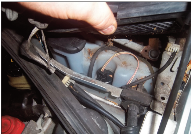
The washer pump on this Clio is easily accessed by unclipping and lifting up the plastic front scuttle panel.
