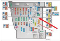
The fuse at position 41 was only 1 Amp and not 25 Amps as it should have been
