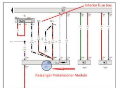
The wiring diagram showed that the noncommunicating SRS Module was supplied power through fuse 41 rated at 25 Amps The technician then checked the power supply into the pretensioner module, as well as the ground terminal. Finally, the LIN bus was scoped to check signal integrity. All proved good, so a new module was fitted and communication attempted. Still no joy.
