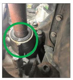
The oil seal had only begun to leak after the clutch had been replaced The new leak on this Picasso was gearbox oil and it was coming from the offside driveshaft seal. As the leak had only occurred after the clutch job, it was pretty certain that the seal had been damaged during the process of replacing the clutch.
