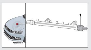
trouble codes, none were present. Can you help? Answer: Yes, we are aware of this fault affecting 1.6 TDi Passat models with CAYC engine code. The cause is due to a faulty fuel pressure regulator control solenoid. Fit a new fuel pressure regulator control solenoid, located on the fuel
