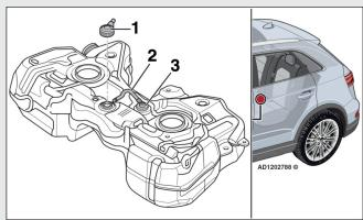
tank breather hose and the fuel tank breather valve for blockages Fig.1.2 & Fig.1.3. If the fuel tank breather hose or the fuel tank breather valve is blocked, fit a new fuel tank. Re-fuel vehicle to ensure fault has been resolved.
