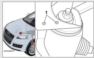
department, to the front subframe using rivets. The deflector plate will help cool the suspension bush. Repeat procedure for opposite side. Carry out road test to ensure noise from
