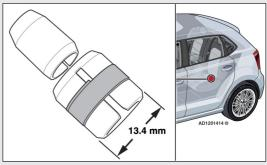
into 6 mm x 55 mm strips. Wrap a new door window glass locating bush, available from Volkswagen parts department, with adhesive tape to a diameter of 13.4 mm Fig.1.1. Fit the door window glass locating bush to the door window glass. Lock the locating bush in place with an expander pin. Refit the rear door window glass. Refit the rear door trim. Repeat procedure for the opposite side.
