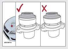
impeller control actuator is stuck in the closed position (see figure above), then fit a new engine coolant pump. This should rectify the fault.
