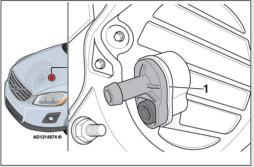
vacuum pump non-return valve (see figure). Check operation of the exhaust gas recirculation (EGR) vacuum control solenoid and replace if necessary. Carry out a road test to ensure the noise has been eliminated.
