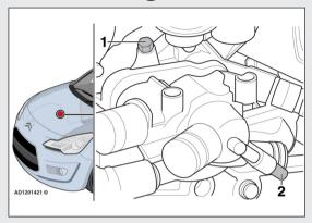
compound (Loctite 9731 60) to the ECT sensor before fitting. Disconnect the thermostat housing wiring harness multi-plug (Fig.1.2). Fit multi-plug of the additional ECT sensor wiring harness to thermostat housing (Fig.1.2). Fit multi-plug of the original thermostat housing wiring harness to the other multi-plug of the additional ECT sensor wiring harness. Secure wiring harness of the additional ECT sensor with cable ties. Carry out road test to confirm the faults have been eliminated.
