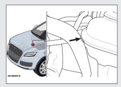
The AC pipe may be contacting the engine coolant expansion tank, at arrow
