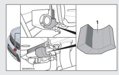
necessary. Fit foam pads, available from Land Rover parts department, to the new engine coolant auxiliary radiator Fig.1.1. Refit front bumper. Ensure front bumper is correctly aligned. Carry out a pressure test on the cooling system after the repair to check the coolant leak
