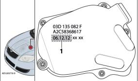
production date is before 06/12/12, replace throttle control unit. This should rectify the fault.
