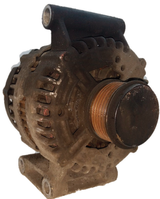
A contaminated and failed alternator
