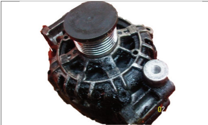
Oil contamination on from bracket of the alternator which enters the alternator from the external source
