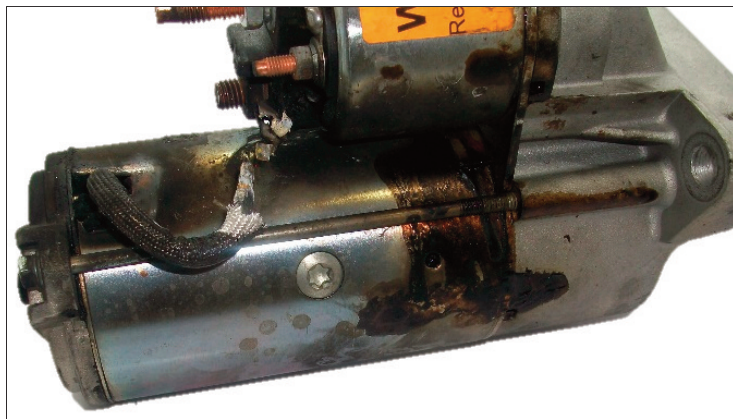
Varnish leaked from starter motor
