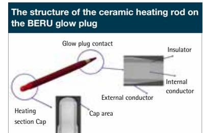
The heating element consists of electrically conductive solid ceramic. Because this has a higher specific resistance at the surface than the supply and return conductor material, the glow rod only glows at the tip (the cap) thus reaching high temperatures faster. The glow plug contact consists of an internal and external conductor with an insulator positioned between them.
