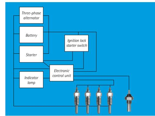
Circuit design principle for a post-heating glow system with four fast-heating glow plugs connected in parallel and a temperature sensor.
