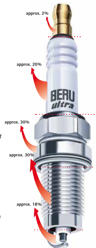
Heat conduction path of a spark plug
