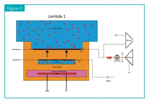
On Toyotas when the engine is running, at Lambda 1 the sensor produces a voltage of 0.3V measured across the sensor. The Electrode B exposed to the atmosphere (air reference chamber – normally negative) is supplied with 3V from the ECM – Electrode A consequently has a voltage of 3.3V (3V + 0.3V). The job of the PID Driver in the ECM is to maintain the 0.3V difference no matter what the oxygen level in the exhaust.
