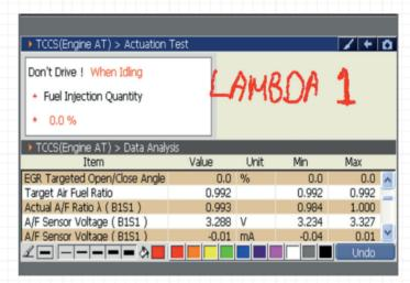
At Lambda 1, sensor voltage is close to 3.3V and no current flows.
