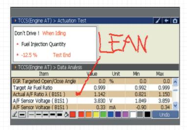
As fuel is reduced the ECM responds by raising the voltage to the sensor and current then flows to the sensor.
