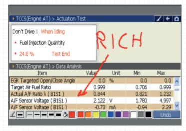
As fuel is added the ECM responds by lowering the voltage to the sensor and the current drains away.
