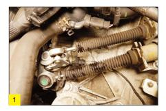
The bell housing bolts located at the top of the transmission need to be loosened and removed, noting the location of each bolt.
