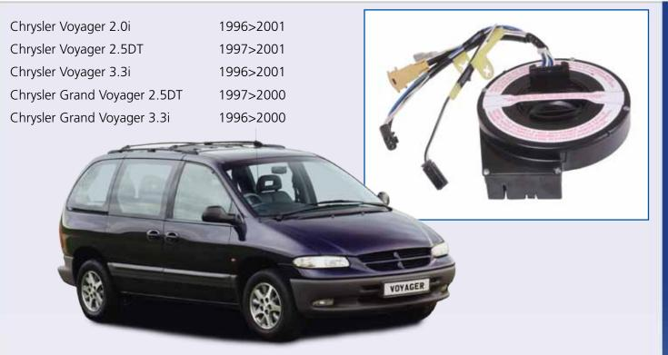
Malfunctioning of the clock spring (also known as Air Bag Squib) on the Chrysler Voyager and Grand Voyager models is not an uncommon problem, to the point that Daimler Chrysler issued a safety recall in the US in 2004 for this particular problem on models manufactured between 1996>2000, which affected as many as 1.2 million vehicles worldwide.
