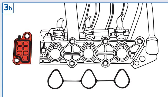
Ensure that the mating surface of the cylinder head is clean and refit the manifold using the new manifold gasket supplied. Fit the new blanking plate onto the cylinder head, using a little RTV if required. Tighten all manifold nuts to the manufacturer's specifications. (15-19Nm)
