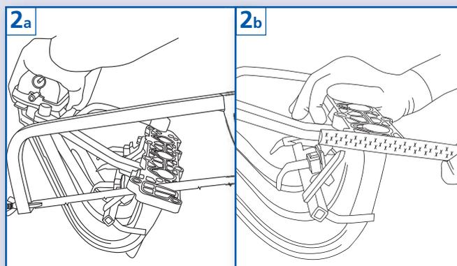
Plug the three outlet ports to prevent debris falling into the manifold. Carefully saw through the manifold and remove the old blanking section. Then trim/file the rough edges of the manifold to ensure a flat mating surface is maintained and clean as necessary
