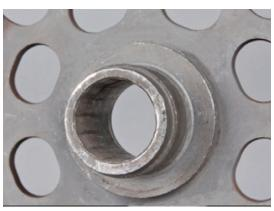
Image 2: Damaged spline profile
