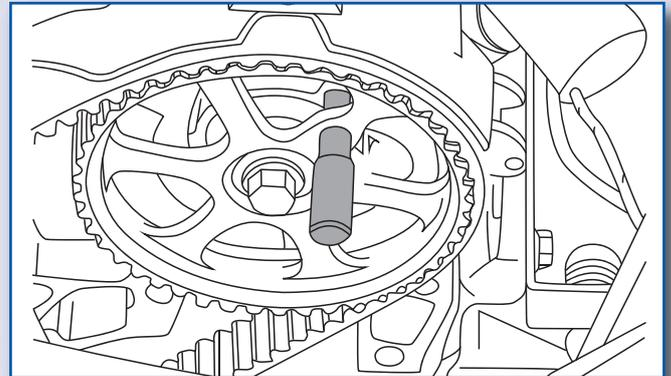
Pin 'B' is used to locate the camshaft sprocket and ensure it does not move during timing belt removal and installation.
