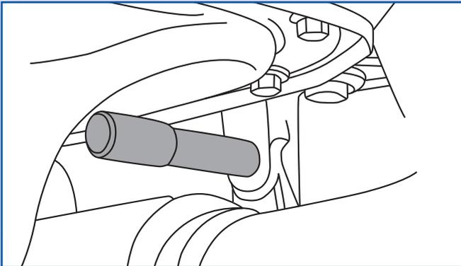
Pin 'A' is used to lock the crankshaft by locating in the back of the flywheel, allowing the crankshaft bolt to be loosened/re-tightened.
