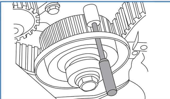
Pin 'C' is used twice during the timing belt replacement process, and is used to align both the crankshaft and injection pump sprockets.
