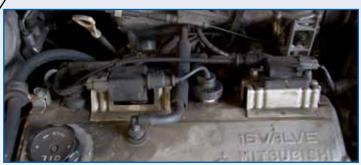
Blue Print strongly recommend that the spark plugs and HT leads are replaced in addition to the coil assembly, or that they are carefully checked. We also recommend that a logical diagnosis procedure is followed (prior to replacing the ignition coil) to prevent it being replaced unnecessarily.
