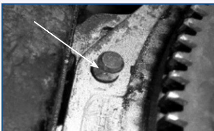
Gearbox location dowels (missing or damaged)
