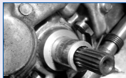
Transmission guide tube wear
