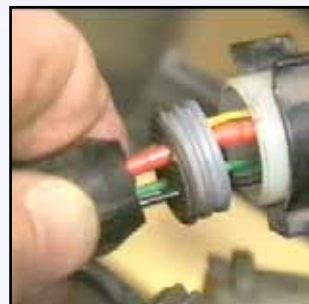
fig 10. - 4-pin connector (bung removed)
