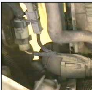
fig 8. - Alternator loom requiring continuity test (inner wing multi plug to alternator)
