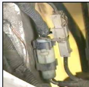
fig 9. - Position of 4-pin alternator loom and main Lucar connector on inner wing
