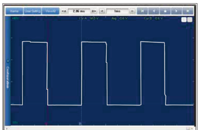
Figure 5 - The SCV duty cycle increased, to try and compensate for loss of fuel pressure, causing the engine to die.
