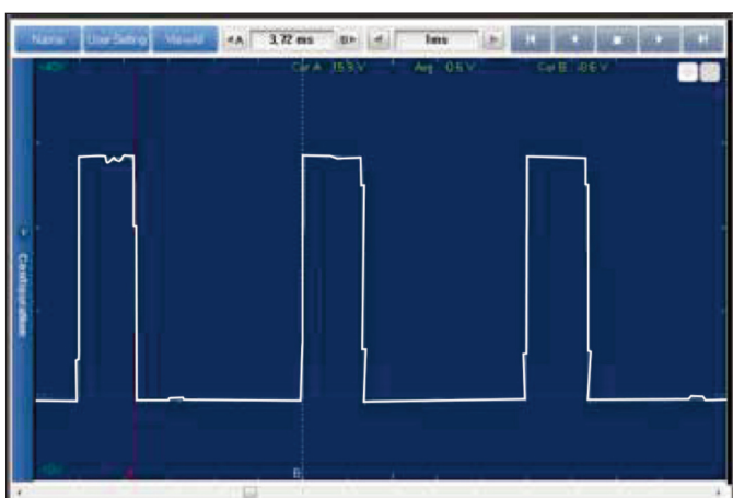
Figure 4 - The SCV duty cycle with the engine at idle
