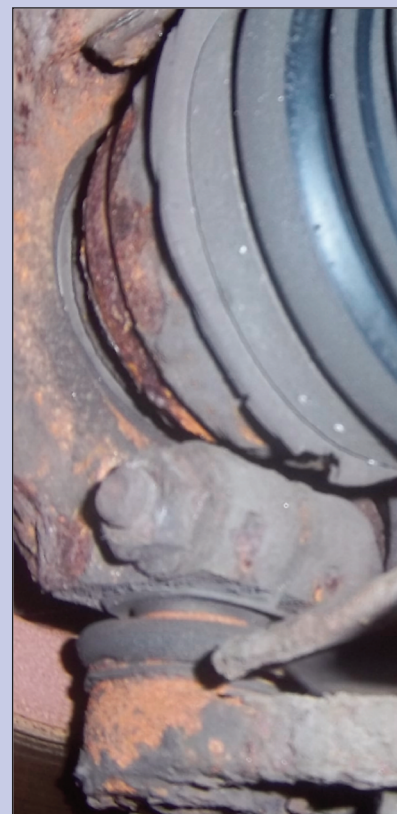
With ABS reluctor ring corroded and the CV boot perished a new shaft was the best option
