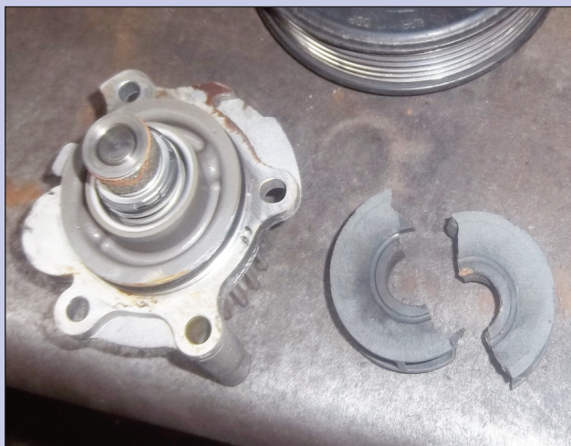
The water pump impeller was in two pieces and providing no movement to the coolant
