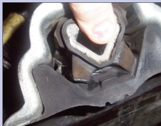
The rubber had begun to crack in the mount allowing excess movement and metal to metal contact
