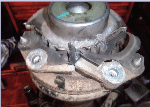
The top mount was not securing the strut to the vehicle, only the van sitting on it had kept it in place.
