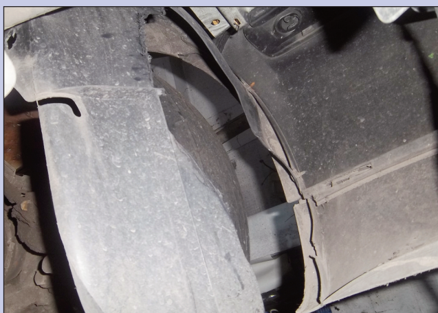
The inner wheel arch had been badly damaged after being dislodged
