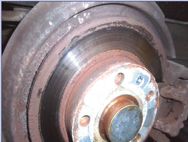
The corrosion around the disc face was causing the poor feel to the brake pedal
