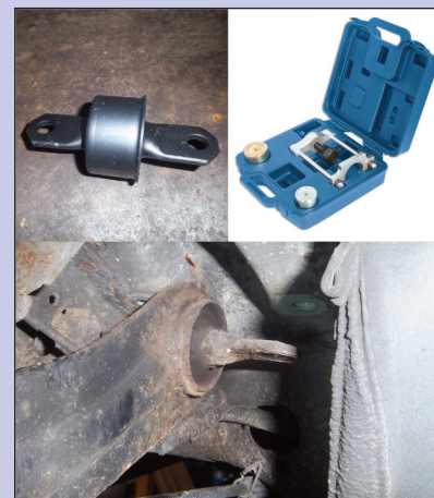
The rear trailing arm front bush is one of the regular test failure points we see on the Focus. Using the correct tool makes fitting a lot easier.
