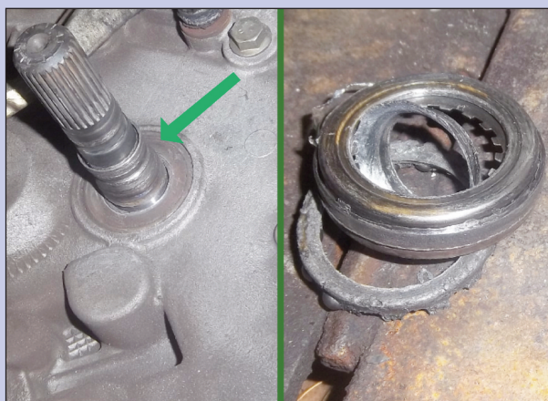
The release bearing had broken to destruction and in doing so had taken out the guide tube
