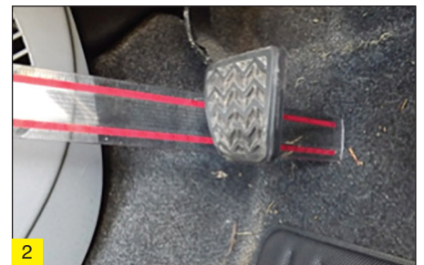
(approx 15-20Nm) until you feel the amount of pressure required increase. Measure the distance travelled by the pedal with a ruler. The amount of free play in the clutch pedal should be 23mm, +/- 5mm (Fig. 2).
