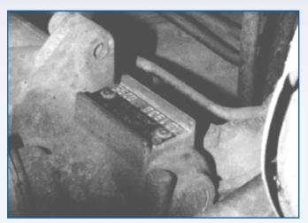
The ZF rack type may be identified by a ZF logo on the green and silver identity plate rivetted into a recess on the front of the steering rack housing.
