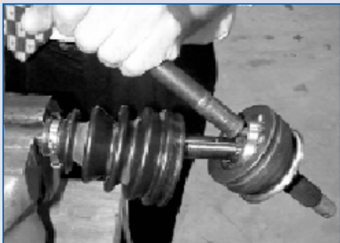
Removal of the original joint
