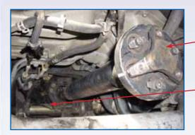
**Driveshaft Coupling (engine side)**
