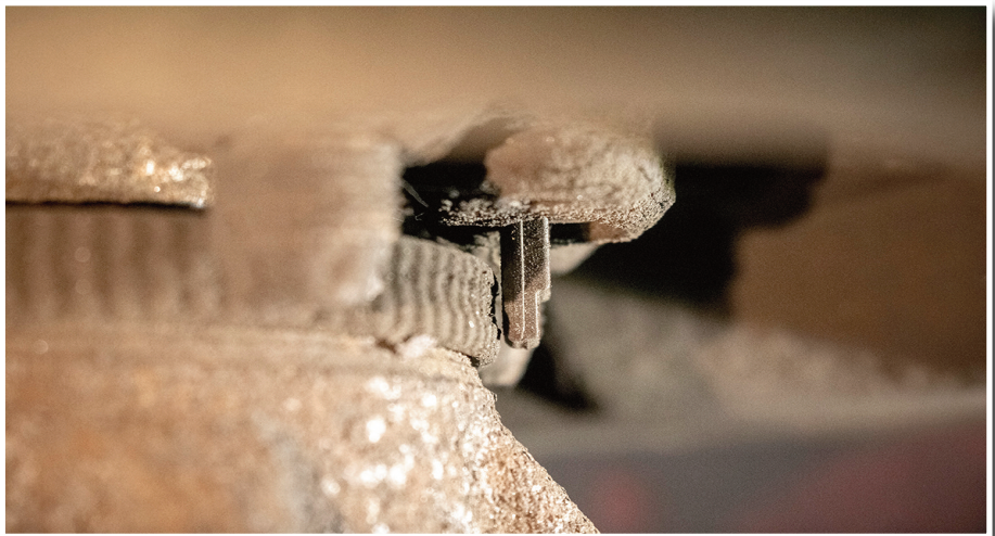
The wheel speed sensors must be aligned with the disc and have a clean, clear gap of 1-2mm (as shown above) to function properly
