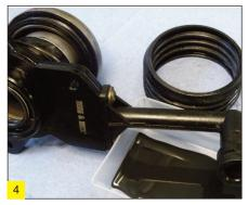
Oil Contaminated Driven Plate (5) Cause Oil leak from gearbox main shaft seal or from engine main bearing seal. Effect Progressing through clutch drag, judder and finally slip. Remedy
