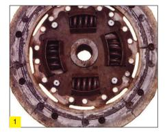
Worn Away Hub Splines (2) Cause Bent first motion shaft or warn gearbox bearings. Effect Loss of drive.
