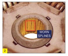
Hung gearbox (3) Cause Gearbox has not been fully installed and left unsupported. Effect Clutch drag due to the damage within the spline. Remedy Replace clutch kit and use a cradle to support the gearbox.
