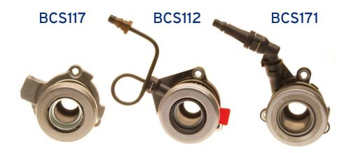
GM is now using a single, modified Concentric Slave Cylinder, which supersedes two older designs.
