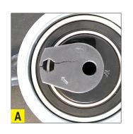
The adjustment cam on the tensioner pulley can fracture during the tensioning process. Continental has provided these instructions for timing belt kits CT1168K1/ K2/ WP1/ WP2/ WP7/ WP9/ K6PRO/ WP8PRO that are for VW, Audi, Seat, Skoda EA288 1.4–2.0 TDi common rail engines.
