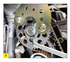
2. Install the new components. In doing so, ensure that for the tensioner pulley, the retaining bracket (Fig 9) sits correctly in the fairing gap (Fig 10). Install the tensioner pulley with tool 303-1054 inserted (Fig 7).
