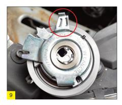
3. Lay the timing belt in an anticlockwise direction starting from the camshaft sprocket: camshaft sprocket, tensioner pulley, crankshaft sprocket, and finally water pump sprocket. Make sure that no kinks form on the timing
