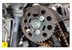
(303-620) must align with the marking on the sprocket.
