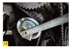
belt during laying. The timing belt must be taut between the sprockets on the pull side.
