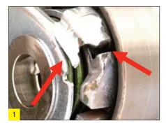
the tension indicator is brought into contact with the hole in the arrester body. As a result, the tension is set far too high and the full load stop is incorporated by the recurring clash with the arrester body until it finally tears or aborts (Fig. 2).
