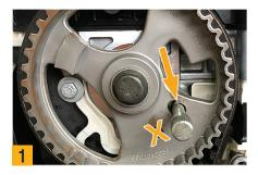
The camshaft sprocket has two locking points: 8mm (Fig. 1) > 1st cylinder TDC for changing the timing belt
