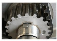
The belt drive is equipped with an oval crankshaft sprocket to reduce power peaks in the belt drive. The crankshaft sprocket is mounted loosely, and can be twisted on the shaft without using the special tool. This, in combination with an incorrectly mounted high-pressure pump, leads to greatly increased force peaks and can cause the timing belt to fail.
