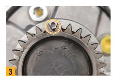
The high-pressure pump itself has markings on the pinion as well as on the housing (Fig. 3), which must be aligned for correct installation. If the high-pressure fuel pump was removed and installed in addition to the timing belt change, first install the timing belt completely and then the highpressure pump
