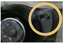
Make sure that it is seated on the pin and that the tensioning pulley lock is not removed until the timing belt has been installed
