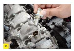
camshaft retaining tool (OE T10120) from the camshaft, turn the engine 360° on the crankshaft in the direction of engine rotation and repeat steps 1–3. If both lock ring tools still cannot be inserted, the timings must be reset. Turn the crankshaft in the direction of rotation, until the marking (keyway) on the camshaft is at the top (Fig. 2).
