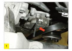
Remove the lower screws of the timing case and then move the coolant reservoir to one side to gain access to the engine mount, which once the engine has been suitably supported from below, needs to be removed, along with the engine mount flange. Then remove the upper half of the timing case, which allows the bottom half to be removed and exposes the timing drive system.
