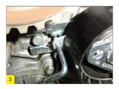
new tensioner, taking care to position it as shown (fig 3). While observing its direction of rotating arrows, install the new timing belt, with its slack section facing the tensioner.
