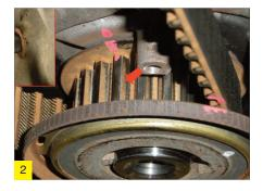
Loosen the bolt on the timing belt tensioner and remove both bolt and tensioner, followed by the timing belt. Replace the idler with the new one from the Dayco kit KTBWP4930 and tighten the nut to 35Nm. Using another suitable pin, hold the fuel injection pump pulley in the correct position and then remove the water pump.
