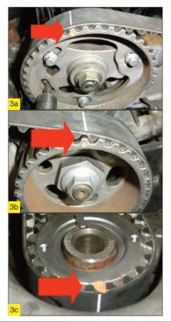
With an Allen key, position the pointer and temporarily tighten the belt tensioner. After checking they are not at the end of the slots, tighten the camshaft pulley bolts to a torque of 15Nm. Remove the camshaft and crankshaft timing tools.
