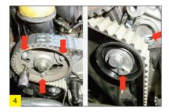
Check that the timing is correct, again by torqueing the camshaft pulley bolts to 15Nm, removing the timing tools and turning the crankshaft clockwise through two rotations and reinserting the tools.
