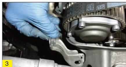
Attach the new idler, Dayco ATB2637 and torque to 45Nm, and tensioner, Dayco ATB2636, ensuring it is fitted as shown (fig 4), and then fit the valve timing units on the corresponding camshafts, but do not fully tighten their screws.
