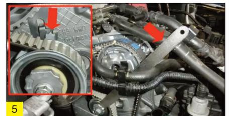
their screws to 50Nm before removing the camshaft timing tools and temporarily refitting the crankshaft pulley to enable the engine to be turned through a few clockwise revolutions.
