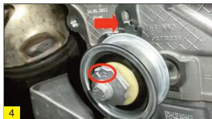
Fit the new timing belt, Dayco 941060, installing it clockwise from the crankshaft pulley via the tensioner, exhaust and then intake camshaft pulleys and the idler. Use the special tool (T10499) to move the needle of the tensioner to the right, about 10mm beyond the fixed reference and then back to the middle of the fixed reference as shown (fig 5). Tighten the tensioner fixing screw to 25Nm.
