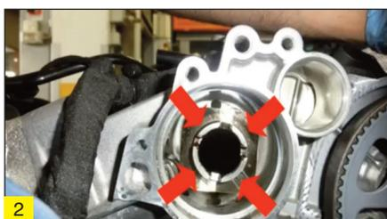
Insert, and fully screw into place, the crankshaft timing tool (T10340) and rotate the crankshaft until the shaft rests on the tool. Then fit the camshaft tool (T10494) and after making sure it is in the correct position, lock it with a screw.
