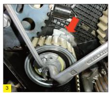
using a 13mm ball-end Allen key, remove the bolt at the back of the auxiliary belt tensioner located under the rear side of the alternator and replace the tensioner with Dayco
