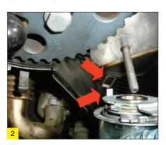
Rotate the belt tensioner with its position index inside the space in the back plate as shown (**Fig 3**) and tighten to 20Nm + 45 degrees.
