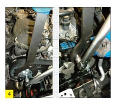
After replacing the timing belt covers and other previously removed components, replace the crankshaft pulley with Dayco DPV1123 and tighten the bolts to 10Nm + 90 degrees.
