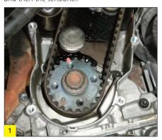
Remove and replace the belt tensioner stud with the new one supplied with the Dayco timing belt kit KTBWP5630, along with the lower and central idlers with nut and bolt respectively.
