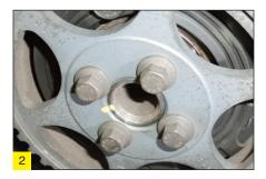
to ensure it is refitted in the correct position, mark its position with paint before removing it (Fig 2). Once the camshaft pulley is detached, take off the idler and then the rear timing belt cover, to allow the removal of the water pump.
