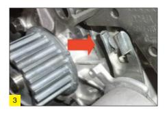
Using the mark painted on earlier, refit the camshaft pulley, followed by the new timing belt, ensuring its correct direction of rotation and leaving the slack section facing the tensioner.
