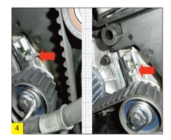
Turn the crankshaft through two rotations and check the engine timing remains correct.
