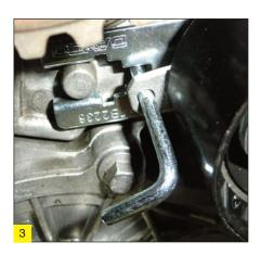
complete with its seal, followed by the new tensioner, taking care to position it as shown (Fig. 3). While observing its direction of rotating arrows, install the new HT timing belt, with its slack section facing the tensioner.
