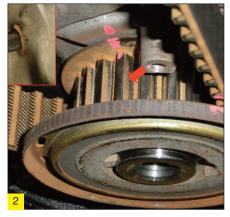
the engine block (Fig. 2). As this is difficult to reach, it is wise to paint a mark on the crankshaft pinion and engine case.
