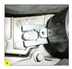
With an Allen key, rotate the tensioner anticlockwise to tension the belt correctly and tighten the bolt to 25Nm. Rotate the engine and check the timing. The correct belt tension has been achieved if the tensioner is positioned as indicated (Fig. 4). Naturally, repeat the process if necessary.
